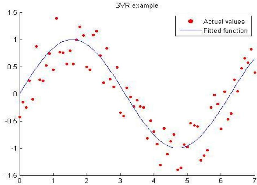
**Figure 3:** A nonlinear SVR case in a 2 dimensional data space
