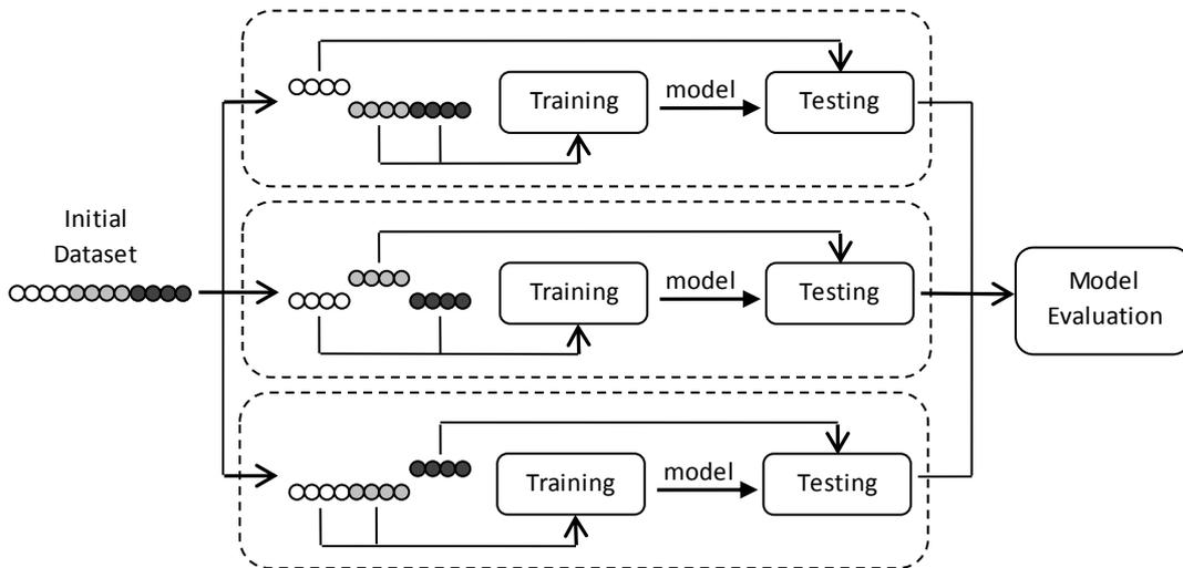
**Figure 5:** Overview of a 3-fold Cross Validation Evaluation System. It shows that each subset is used as a testing sample while the others are used for training the model.
